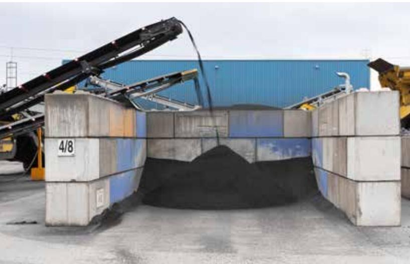
ALFA SINSTONE®, GRIPSTONE® and SICILYSTONE are by-products obtained from the recovery of black steel mill slag composed mainly of iron, calcium and silicon oxides, which is generated during the melting process of ferrous scrap in the electric arc furnace. These are high-performance artificial aggregates resulting from continuous research into new materials and new technologies for improving manufactured products and safeguarding natural resources.
